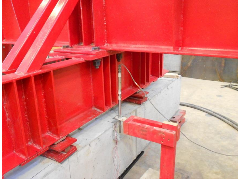
Figure 4.15: LVDT Set-Up for Beam Splice Test
