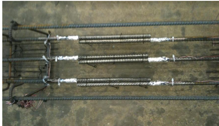
Figure 4.9: Spliced Length with Attached Strain Gauges
