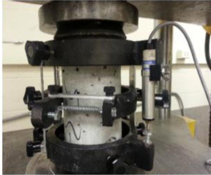
Figure 4.6 Modulus of Elasticity Test Setup
