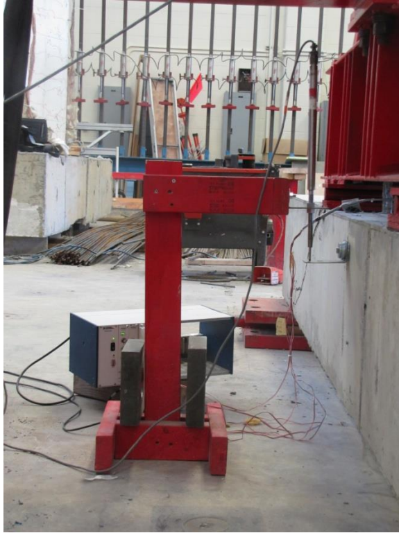
Figure 4.10: Detail of LVDT for Deflection Measurement
