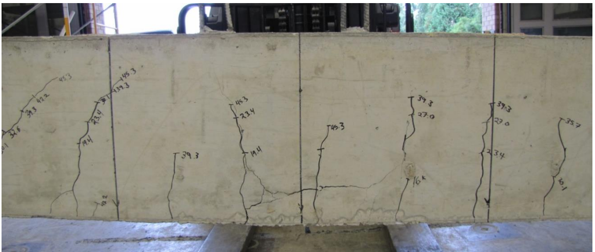
Figure 5.13: Beam Splice Crack Propagation at Failure (RAC50-1)
