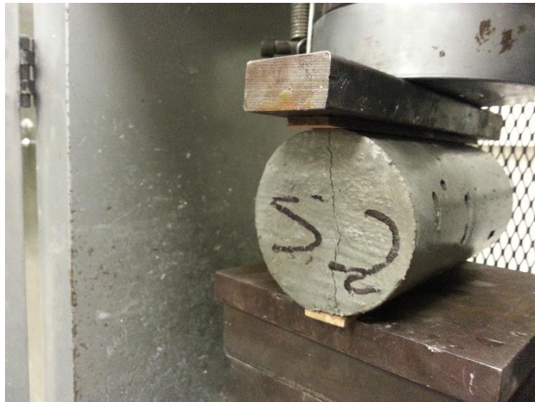
Figure 4.4 Splitting Tensile Strength Test Setup
