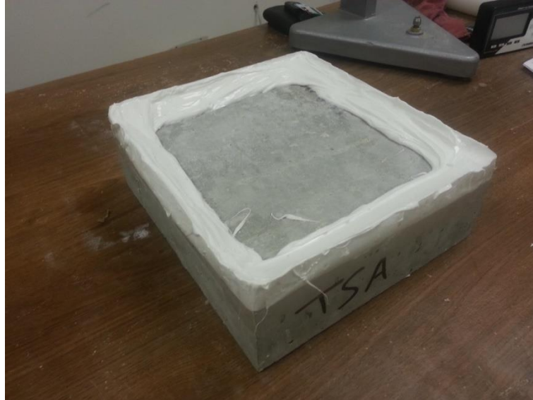
Figure 4.18 Silicon made Dike for Ponding the Surface of the Specimen with a Chloride Solution
