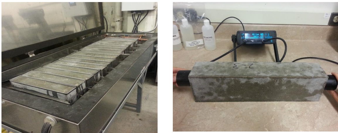
Figure 4.20 Freeze/thaw Testing, Procedure A, Freezing and Thawing in Water (left); Measurement of Pulse Velocity (right)
