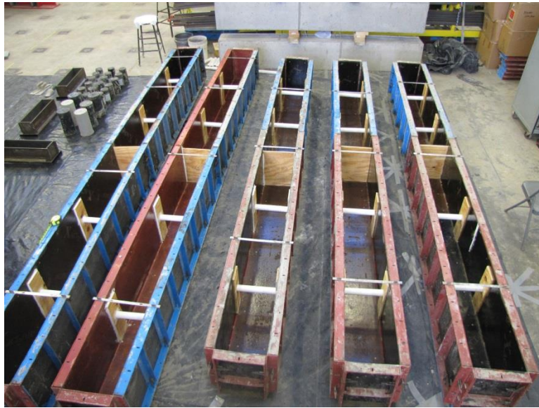
Figure 4.1: Formwork for Casting Pre-Recycled Concrete
