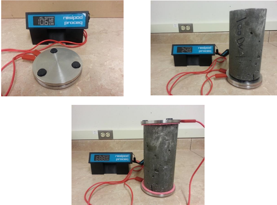
Figure 4.13 Measuring Bulk Electrical Resistivity. Top Foam (top left), Lower Foam (top right), and Specimen Resistivity (bottom photo)
