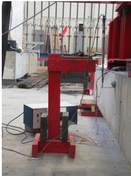
Figure 3.9: Detail of LVDT for Deflection Measurement
