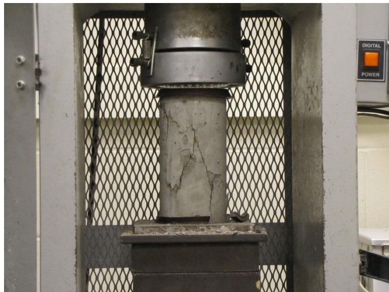
Figure 3.1: Compressive Strength Test
