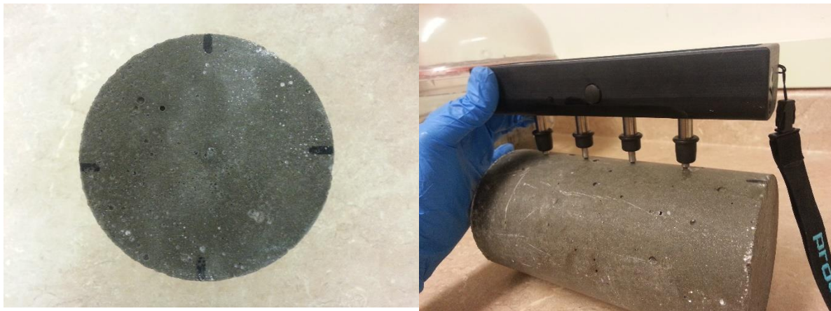
Figure 4.11 Surface Resistivity Measurement
