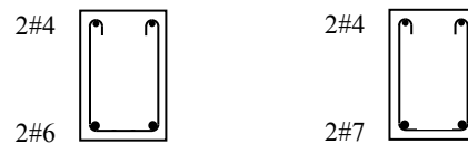
Figure 3.1: Cross Sections and Reinforcement Layout of the Beams
