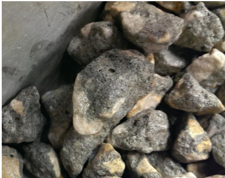
Figure 5.4: Close Up View of Washed RCA
