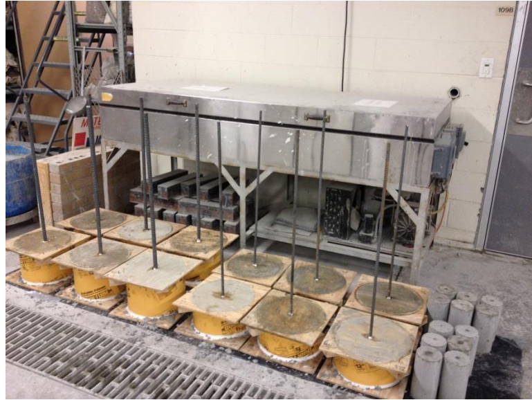
Figure 4.4: Completed Direct Pull-Out Specimens in Molds
