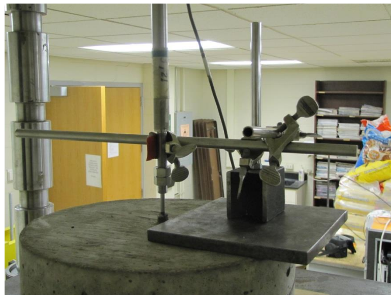
Figure 4.6: LVDT Set-Up for Direct Pull-Out Specimen
