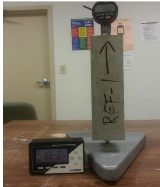
Figure 4.8 Measuring the Length of the Shrinkage Specimens
