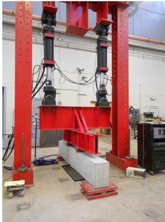
Figure 4.14: Beam Splice Specimens in Load Test Frame
